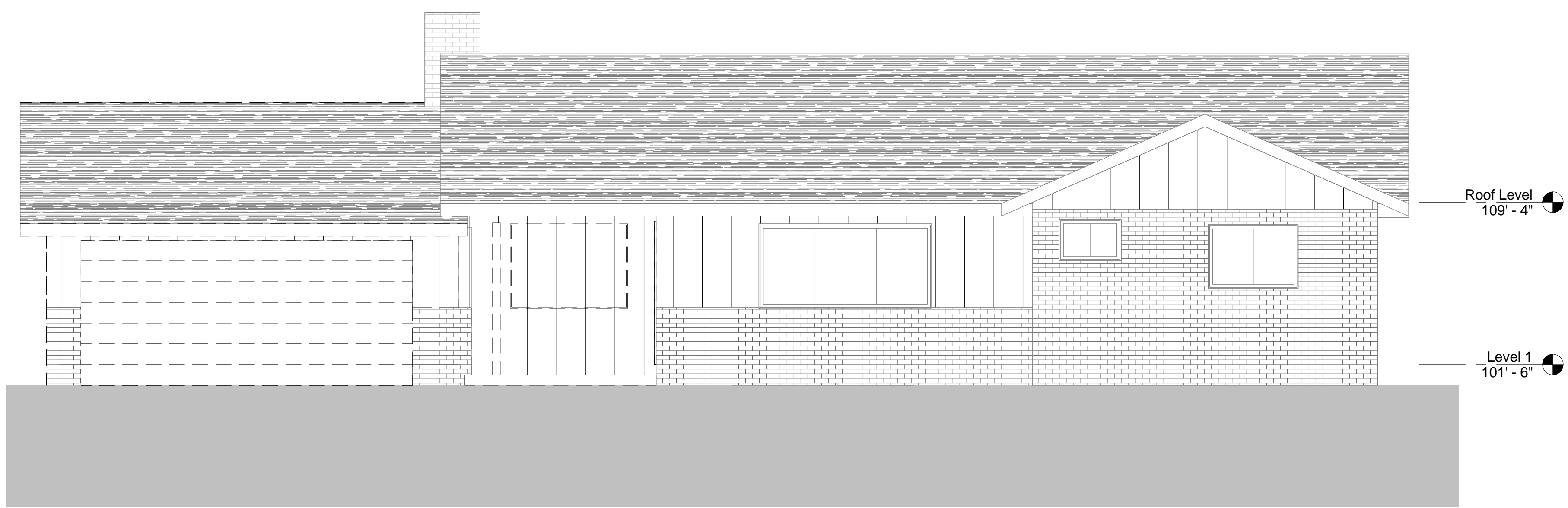
2 Front (East) Elevation - Existing 1/4" = 1'-0"
